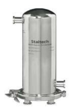
Designed for environments where the cooling water supply may lead to fouling of the coil, the HSC50 can be disassembled for cleaning. The orientation of the sample connections also makes the HSC50 suitable for continuous in-line cooling applications such as conductivity monitoring in high purity systems.
