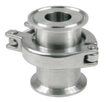
The HCV04 range is ideally suited to steam, condensate and process fluid applications. Standard valves have metal-metal seating and a choice of 8 or 35 mbar opening pressure. A range of soft seat options are also available. Wetted surfaces on all valves are finished to 0.5 microns Ra
