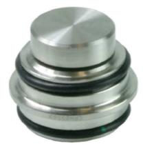
The HCV01 check valve is designed to fit , between two ASME BPE compliant clamp fittings, sealing on the ID of the tube using FDA approved EPDM O-rings. The compact 316 stainless steel design is suitable for a wide range of duties in steam liquid and gas service, including pressure relieving and anti-vacuum applications. Standard valves have metal-metal seating. A number of soft seat seal and spring options are also available
