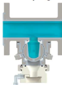
SSB Flanged 1.4408-PFA with vertical adapter and pneum. actuator
